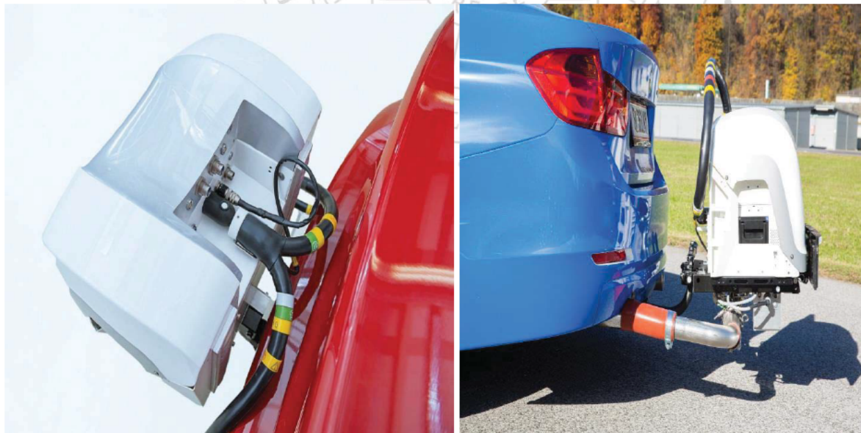
Figure 3. Typical trailer hitch installations of AVL system with enclosure
